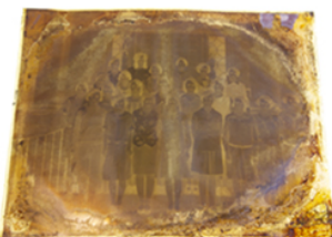
Level 4 The film becomes an amber color and the image begins to fade.
