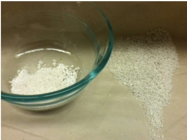
Grated vinyl eraser crumbs before and after surface cleaning. Credit: Jackie Divis Doyle, Binding Obsession 01-23-2012
