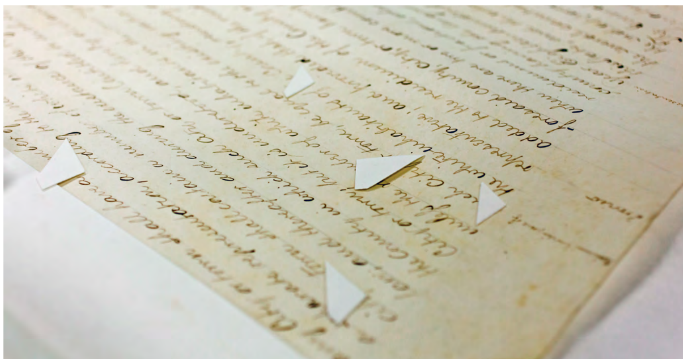
Areas of friable media marked with blotter triangles.
