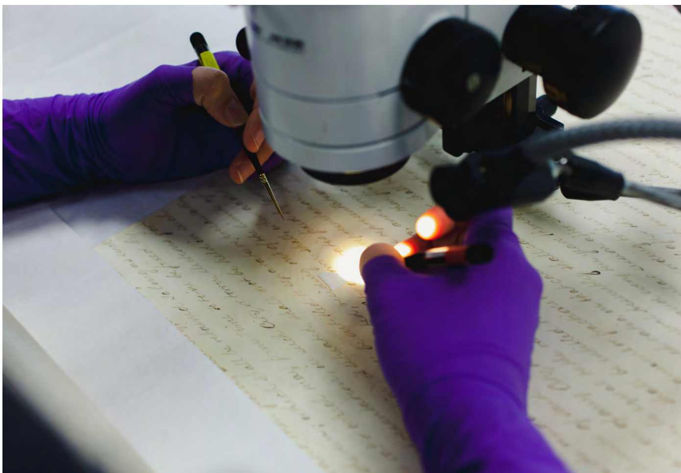
Conservator working at the microscope to apply ethanol and gelatin with a two-brush technique.
